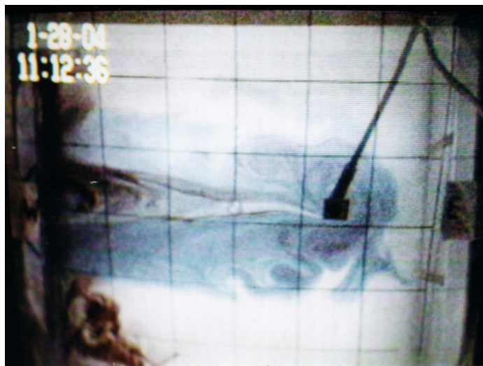
Figure B-2: A photograph of the steady state circulation pattern (visualized by colored dye) that shows a zonal jet at the latitude of the forcing flanked by a pair of counter-rotating recirculation gyres consistent with the numerical simulations.
