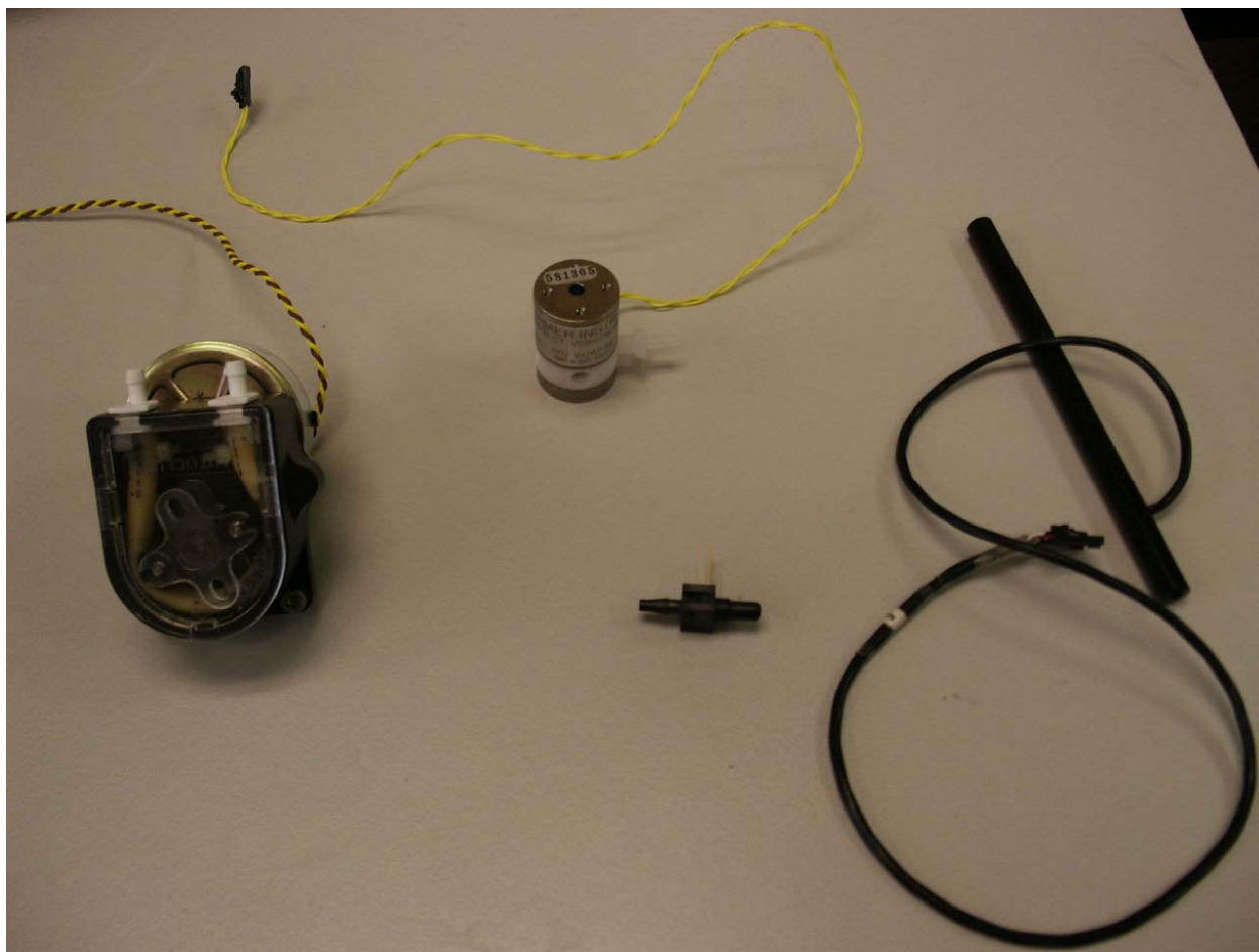
Figure 2. The major components of the fluid system – clockwise from left: peristaltic pump, solenoid valve, 545 CT cell (with custom connector installed), DP cell (before installation of custom circuit board).
