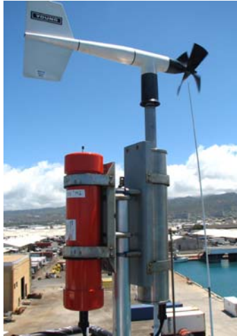
Figure 5. AutoIMET system installation on the Kilo Moana . The met tower (upper photo) is above the bridge, about 20 m above the water line. The logger box with BP, and the sensor box with AT/RH and radiometers, were installed on pipes on the port side of the tower (lower left). The anemometer and GPS system were installed near the centerline at the stern of the tower (lower middle). The PRC sensor was installed on the starboard side of the tower, just inboard of the ship's sensor (lower right).
