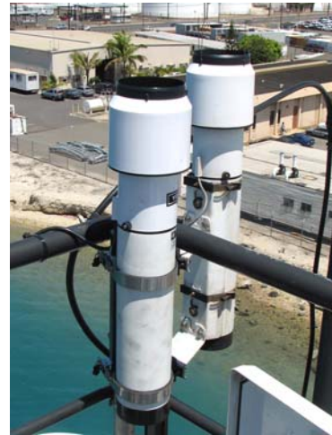
Figure 5. AutoIMET system installation on the Kilo Moana . The met tower (upper photo) is above the bridge, about 20 m above the water line. The logger box with BP, and the sensor box with AT/RH and radiometers, were installed on pipes on the port side of the tower (lower left). The anemometer and GPS system were installed near the centerline at the stern of the tower (lower middle). The PRC sensor was installed on the starboard side of the tower, just inboard of the ship's sensor (lower right).
