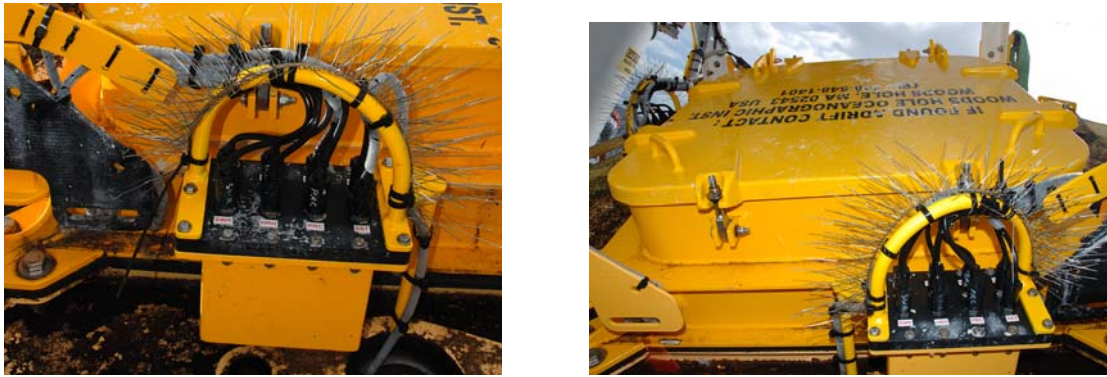
Figure 27: WHOTS-3 recovery with bird wire.
