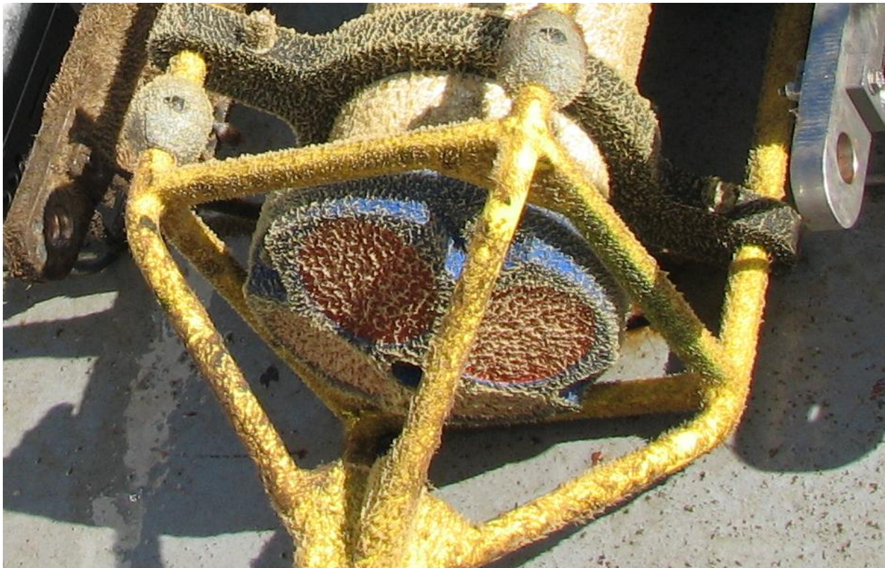
Figure 22. WHOTS-3 ADCP deployed at 125 m after recovery.
