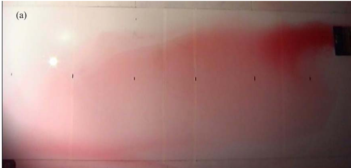
Figure 2. Top view photographs from the 3 regimes. The black marks on the middle of the slope are 1 m apart. The color variation from weaker, on the left side, to stronger on the right side, may be due to a non-uniform illumination. a) Laminar regime, b) Waves regime, c) Eddies regime (the plume is here steered downslope by a canyon) d) Instabilities forming alongside the ridge wall.
