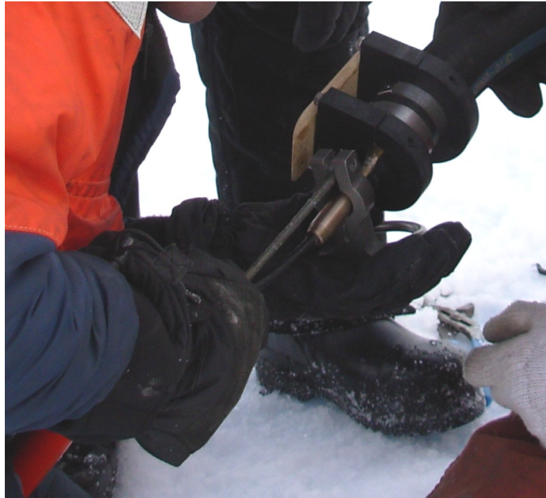
Figure 12: Attaching slip bale to cable.
