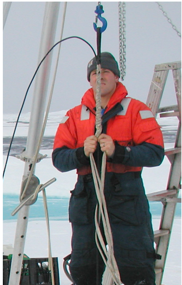
Figure 13. A ‘Yale Grip’ is used to slip the mooring until the slip bale is adjacent to the ‘Yale’ grip.
