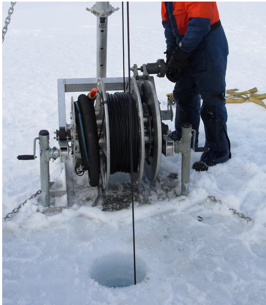
Figure 8: Correct positioning of the winch and brake operator in relation to the deployment hole.
