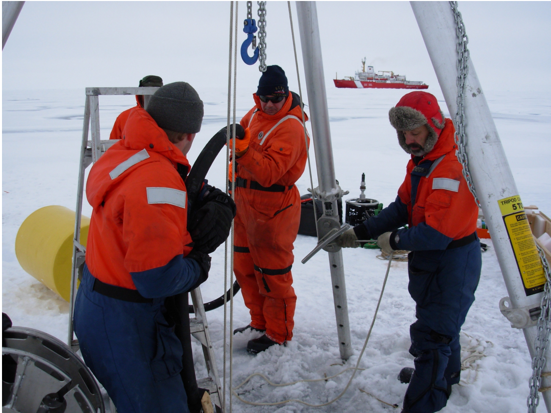
Figure 14: Using the cleat to slip the final section of the mooring into place. The rope at the cable end loops through the slip bale connection on the cable.
