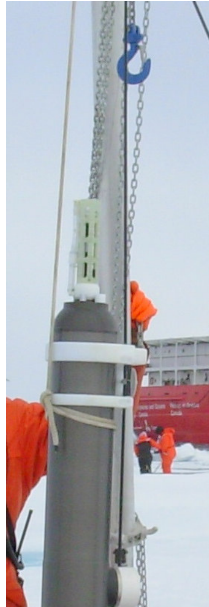
Figure 10: Clove hitch placement for supporting the ITP on the wire rope.
