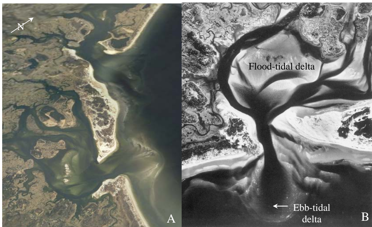
Figure 16. A. Oblique aerial view of the Merrimack Embayment barrier island and tidal inlet system in northern Massachusetts. B. Vertical aerial photograph of Essex Inlet, MA shown in bottom of accompanying photograph.
