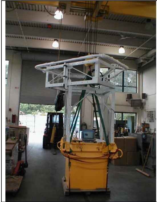
Figure 17: S8 Rigging of the assembled buoy for buoy spin (or ‘hard-iron calibration’)
