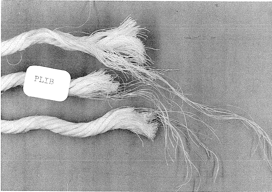
Figure 2.6 Parted mooring line (washed and dried).
