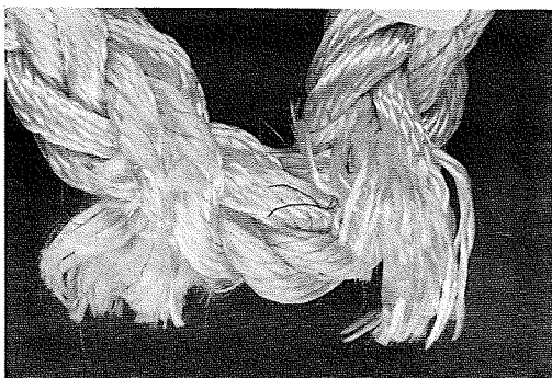
CAUSE OF DAMAGE — UTILITY KNIFE BLADE
