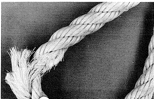
CAUSE OF DAMAGE — UTILITY KNIFE BLADE
