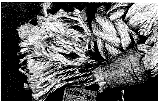
CAUSE OF DAMAGE — WIRE CUTTER
