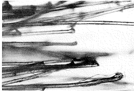
CAUSE OF DAMAGE — POCKET KNIFE
