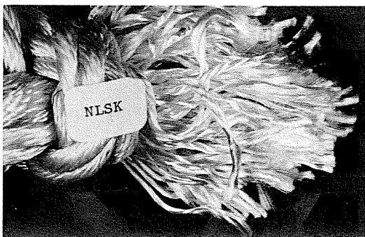
CAUSE OF DAMAGE — POCKET KNIFE
