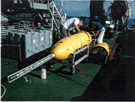
(a) An AUV with a single line array.
