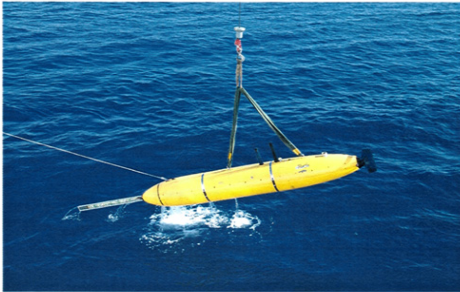
Figure 2-2: An Odyssey-III AUV. This survey-class AUV is able to carry a wide variety of scientific sensors and is able to operate underwater unattended for long periods of time.
