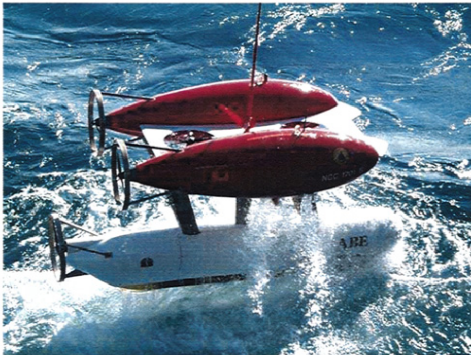
Figure 2-3: The Autonomous Benthic Explorer (ABE). ABE can survey the ocean floor at depths up to 5500 m carrying a variety of sensors such as cameras, sonar, and chemical sensors. ABE is operated by the Woods Hole Oceanographic Institution.
