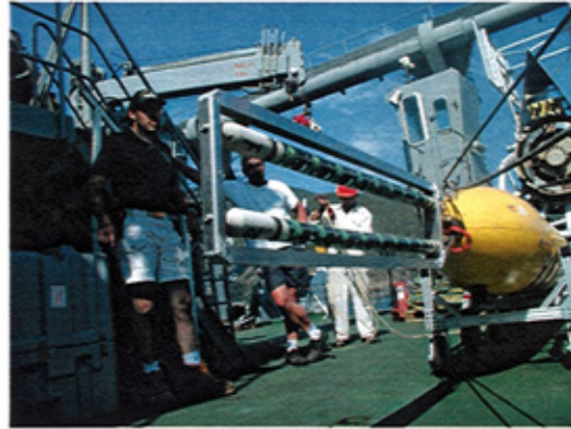
(b) An AUV with a dual line array.
