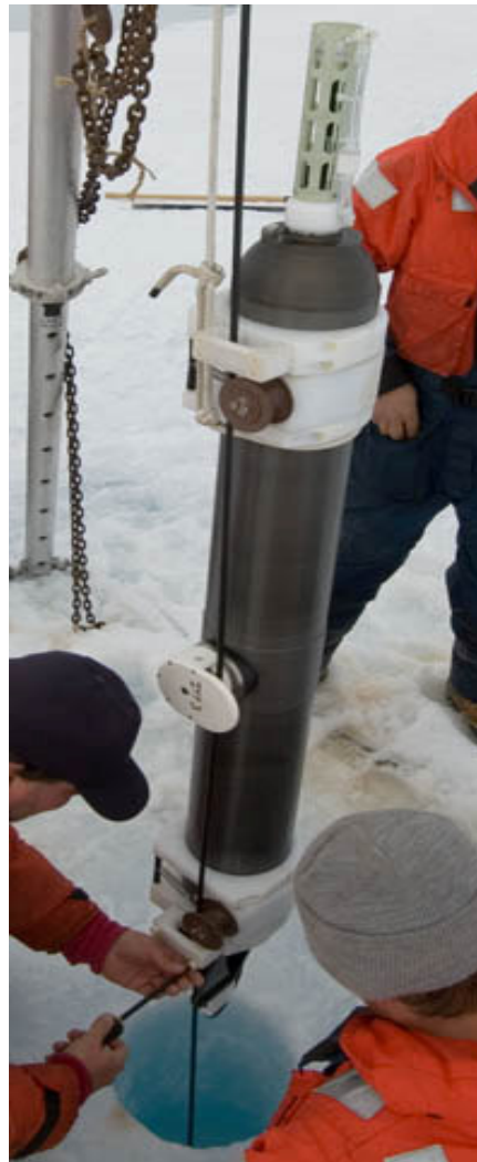
Figure 7: Attaching ITP to mooring wire during deployment.
