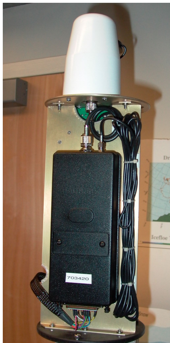
Figure 5. NAL Iridium modem and antenna on ITP electronics chassis.
