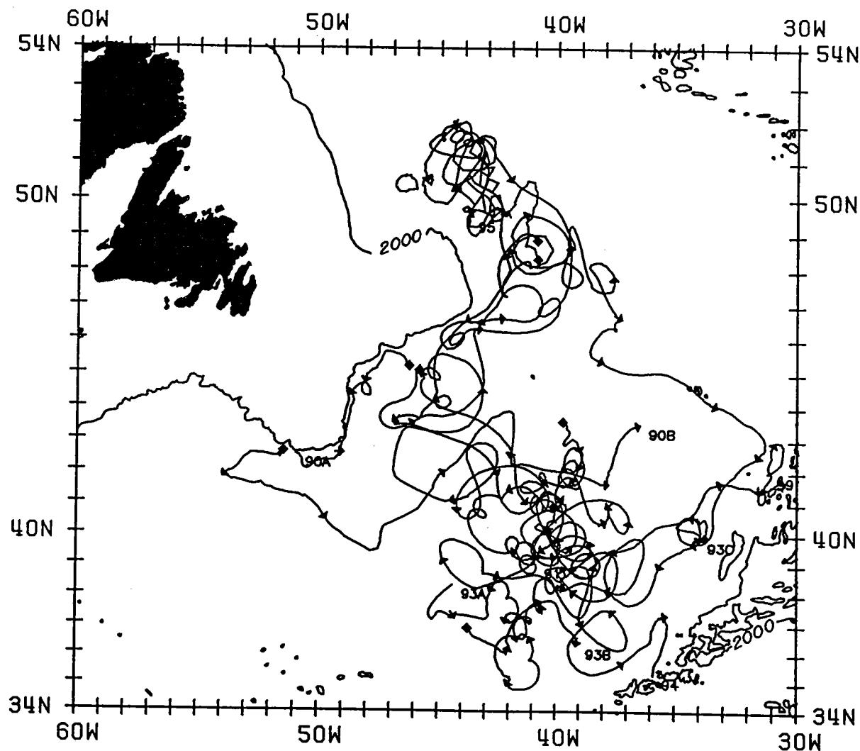
Figure 5: A composite of six float trajectories at 700 m between 1986–1989.
