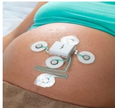
FIGURE 6 The Monica AN24 (left) with real-time FHR extraction uses discrete electrodes. The Novii on the right shows the improved package, which incorporated all of the IP from the AN24 into the small pod (white module) but with electrodes now delivered on a single PET substrate offering a truly wearable foetal monitor
