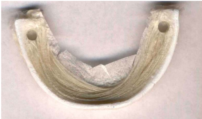
Figure 1. Photograph to show fibre orientation in the scaffold.
