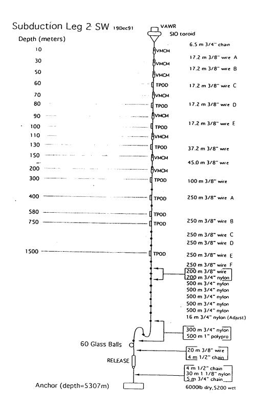
The following morning the slant range to the release remained at 2747 meters. After ranging on the acoustic release a release command was sent. To our surprise, confirmation of release was received and the tension dropped to 4000 pounds. Fortunately the anchor dropped away and the recovery tensions dropped to something more manageable. The ship immediately put some way on so as to move the ship out of the way of the rising glass balls. The glass balls surfaced about a mile aft of the ship.
