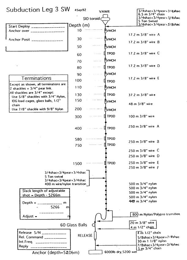
fell to the bottom, the temperature went out of the instrument's measurable temperature range. All five SIO temperature recorders collected data up to the time the mooring failed. Seven SIO VMCMs were recovered. With the exception of one VMCM which had a tight propeller, all the others appeared in satisfactory mechanical condition. All instruments, except the 10 meter VMCM, were recovered.
