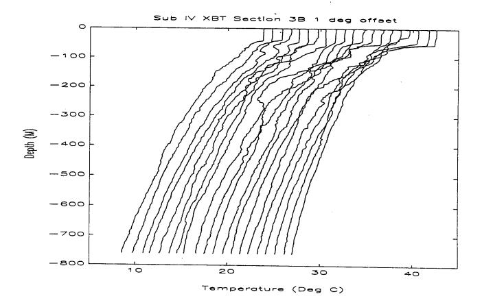
Figure A8-4f Overplot of XBT Profiles 115 to 121, 123 to 128, and 130 to 136. Successive profiles are offset by 1°C.
