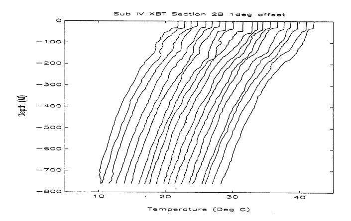
Figure A8-4d Overplot of XBT Profiles 69 to 89. Successive profiles are offset by 1°C.
