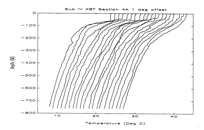
Figure A8-4g Overplot of XBT Profiles 137 to 156. Successive profiles are offset by 1°C.
