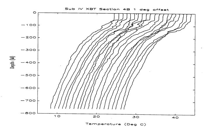
Figure A8-4h Overplot of XBT Profiles 157 to 167. Successive profiles are offset by 1°C.
