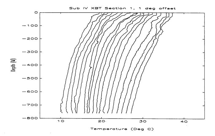
Figure A8-4b Overplot of XBT Profiles 25 to 45. Successive profiles are offset by 1°C.
