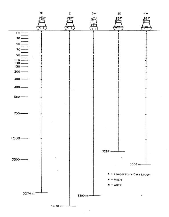
Figure 4. Subduction 3 Northwest Mooring Schematic
