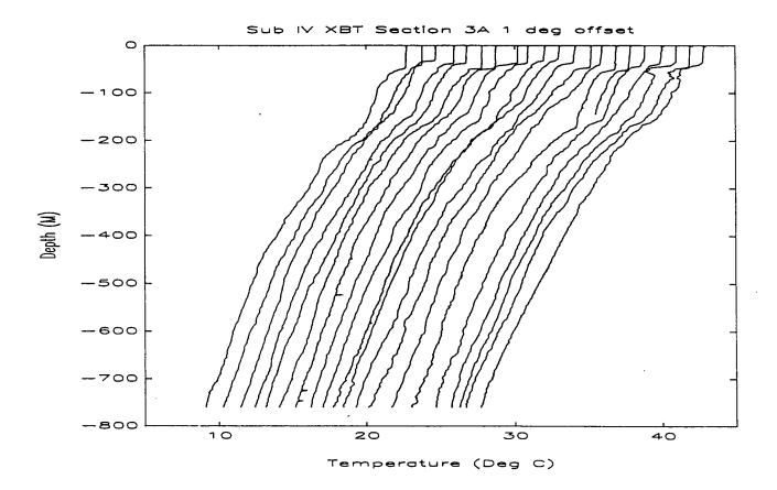
Figure A8-4e Overplot of XBT Profiles 91 to 94, 97 to 100, 102 to 107, and 109 to 114.
