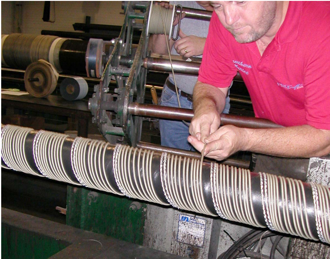
Figure 4. Constructing compliant stretch hose around a mandrel. After the initial rubber and cords are assembled, the electrical conductors shown being helically wound around the hose before the final layer of rubber is applied and the whole hose cured.
