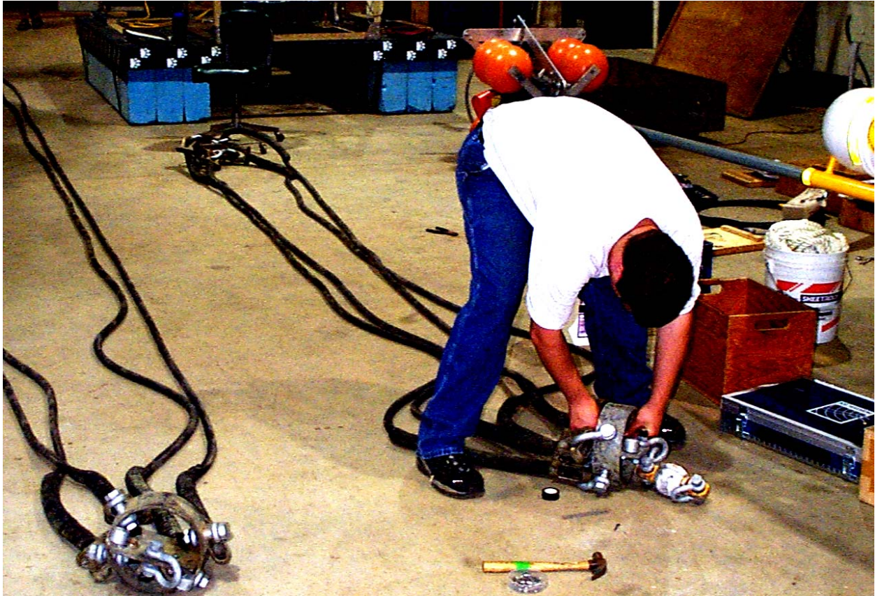
Figure 6. Compliant Tether Assembly. Four elastic tethers are attached to bridle assemblies at each end. A swivel prevents the tether assembly from becoming twisted (seen on the bridle assembly on the right). These two tether assemblies are used on the environmental monitoring mooring deployed off New Hampshire (see Figure 9).
