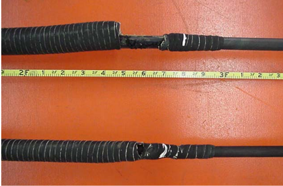
Figure 33. Detail of the splice slip in the tethers after the 3000 cycle extended test.
