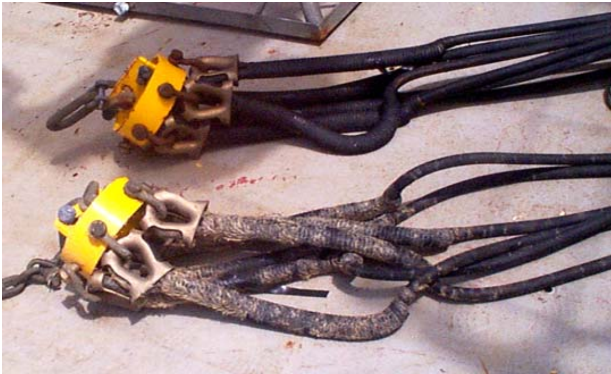
Figure 7. Two six-element elastic tether assemblies after six months deployment on Georges Bank in GLOBEC. The top is from the Northeast Peak and the bottom from the Southern Flank. The mooring configuration for both tethers is shown in Figure 9. The splices in the top picture show no curving due to over tensions, but the bottom ones show a little slippage, but the tethers were successfully redeployed. Only a little biofouling is observed on each assembly.
