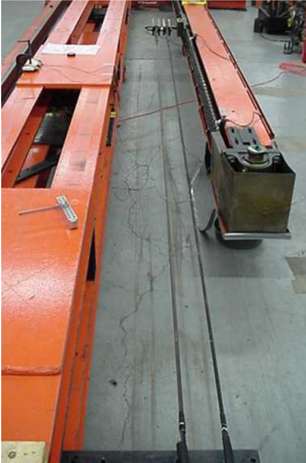
Figure 19. The tethers undergoing tests in the machine. The far end (crosshead) moves back and forth with the chain drive.
