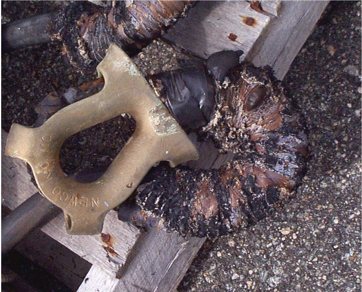
Figure 13. A tether from GLOBEC that has been pulled so that the splice slipped. When the tension was removed, the splice curled up in a 360-degree circle. The tether rubber, remains under high tension around the thimble. This splice was then left out in the sun and weather for a year, and shows the degradation of the rubber tape with sunlight.
