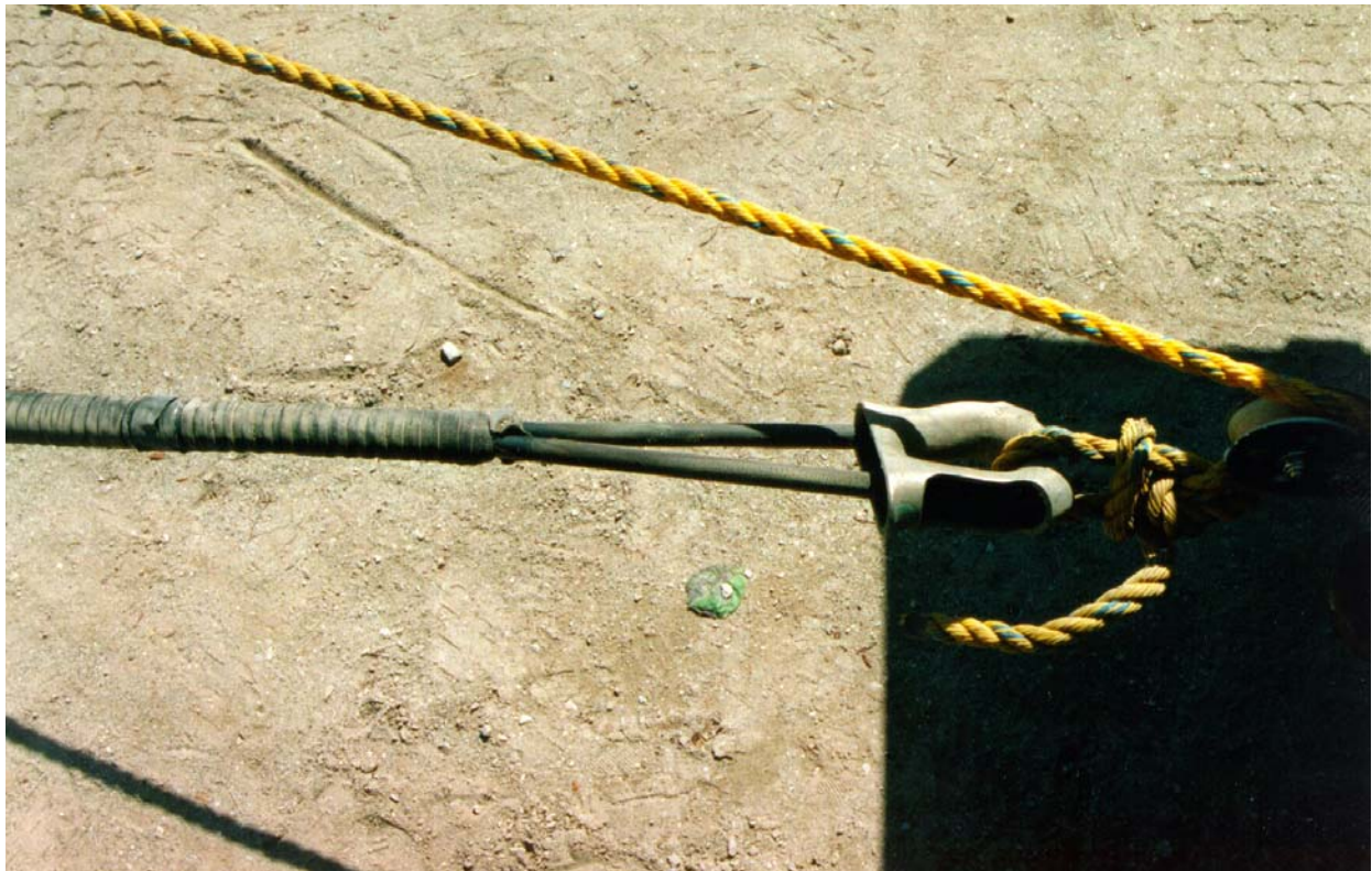
Figure 12. Elastic tether stretched to about 500% showing the stretch of the splice, and the thinning of the elastic under tension. This is a GLOBEC tether after a year of deployment with slight checks observable in the rubber. In this case, the checks did not degrade the performance of the tether.
