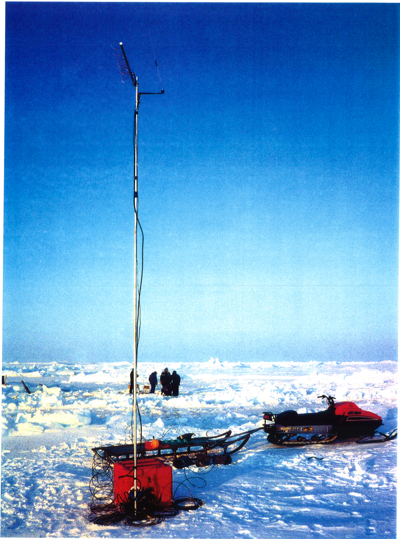
Figure 4. Photograph showing one of the RLAM deployments during SIMI-94. Note the directional looped YAGI for the 902-928 MHz LAN and the 3 dB omni for the UHF "survival" link.
