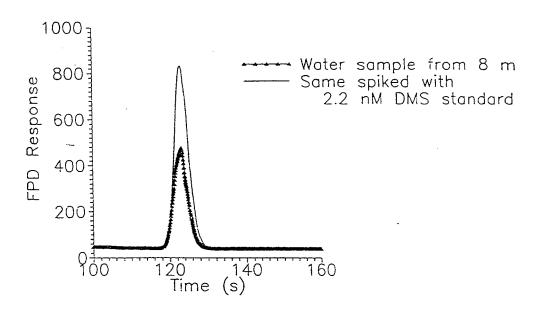
Figure 2: Chromatograms showing detector offset as a function of time for a water sample before and after a 2.2 nM DMS standard addition
