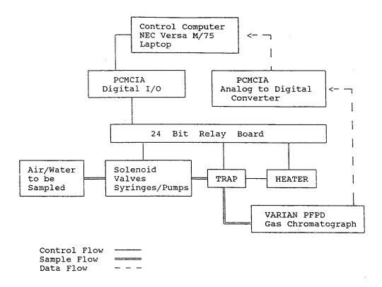
Figure 1: Unattended Trace Gas Measurement System
