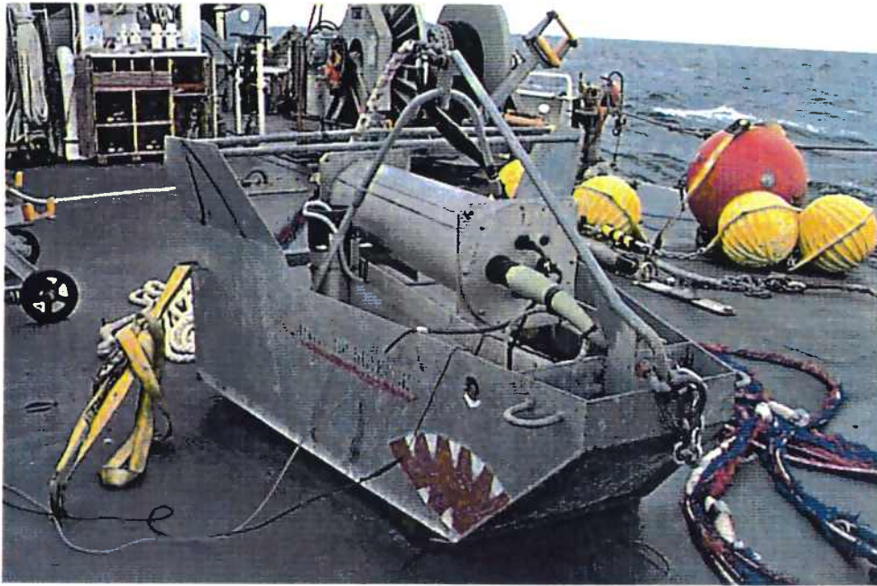
FIGURE 58. The “Shark of Science” anchor containing storage electronics.
