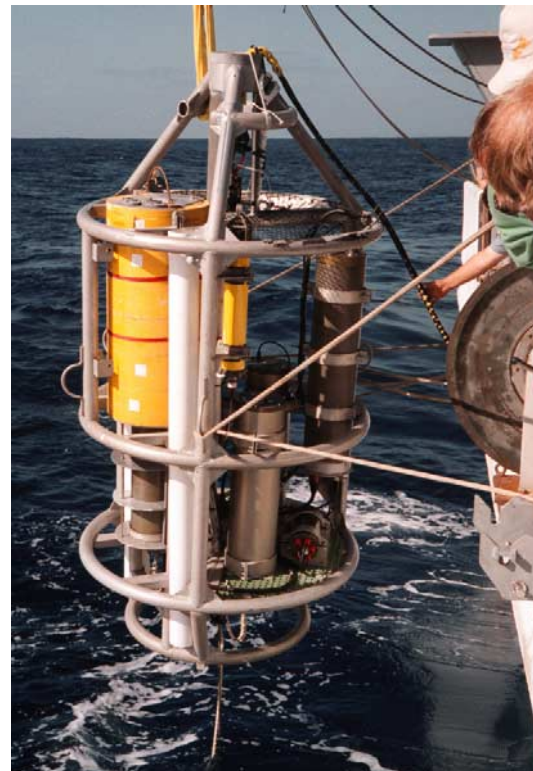
Figure 6. The bottom instrument package consists of a frame that is designed to sit in the reentry cone. It contains the bottom control unit (the gray housing in the upper right), the data recording unit (in a sleeve of yellow syntactic foam on the left) and three large housings of lithium batteries (one of the battery housings can be seen in the lower foreground). Above the battery housing is one of two yellow acoustic transponders.
