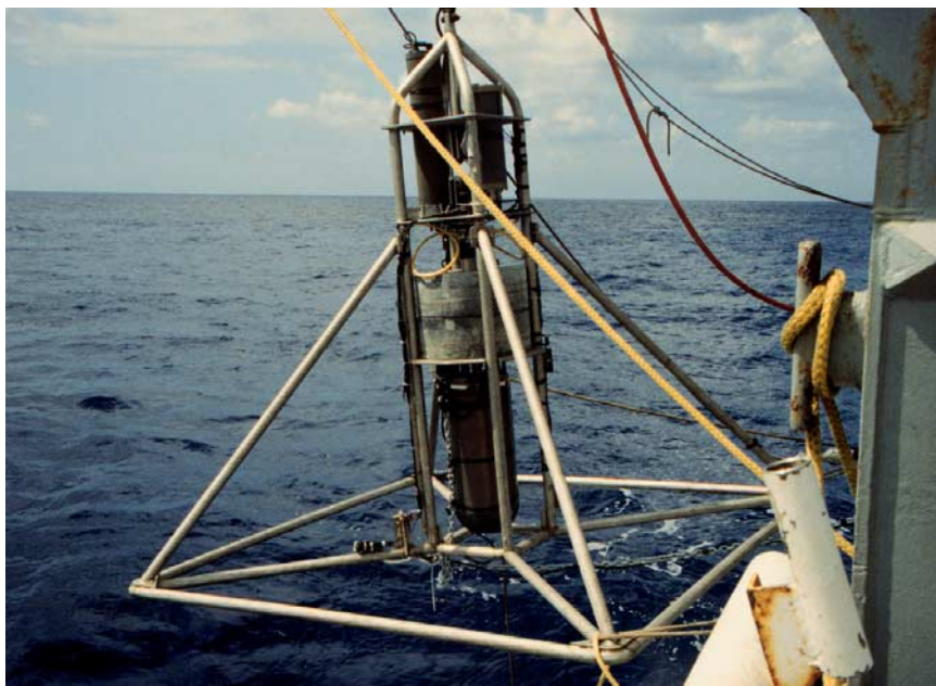
Figure 11. The buried BBOBS seismometer is shown in the burial frame as it is deployed off the fantail of the R/V Thompson. The burial system is described further in Wooding et al. [2001].
