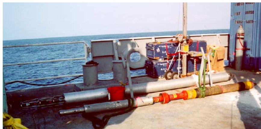
Figure 13. The borehole packer system was intended to block fluid flow in the hole that might cause noise on the borehole seismometer. As configured for deployment by the wire line reentry system it consisted of two units. The lower unit with the packer, its setting tool, hydraulic pump, motor and pressure gauge is in the foreground with the yellow and red sections. Behind it is the upper unit with the lead-in package and a reservoir of hydraulic fluid for expanding the packer. The lead-in package (LIP) can be seen to the left of the hydraulic unit. This system was tested during the OSNPE.
