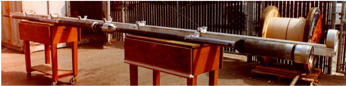
Figure 12. The reentry probe (also called the logging tool) used to test the hole prior to installation of the borehole seismometer is shown. Its components are: a low light level TV, 80 watts of illumination, two three arm calipers, a platinum resistance thermometer, a pressure gauge and a navigation transponder.
