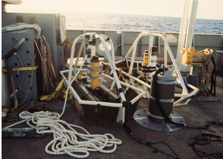
Figure 10. The seafloor BBOBS (Broadband Ocean Bottom Seismometer) is shown next to the two DARS (Data Acquisition and Recovery System) frames on deck. The white rope is the soft tether which accommodates heave after landing the package on the seafloor.
