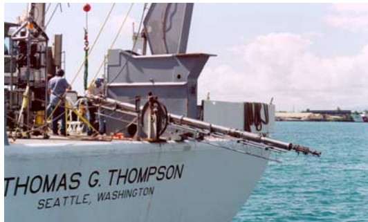
Figure 5. The borehole seismometer was deployed from a “teeter-totter” on the fan tail of the R/V Thomas G. Thompson. The lead-in package (TV, lights and navigation transponder) is about 2 m long and can be seen at the right at the end of the seismometer. Three clamping arms were used at the top and bottom of the seismic sensor package to lock the seismometer into the casing. The seismic sensor package consists of a Teledyne KS54000 in a titanium pressure housing.
