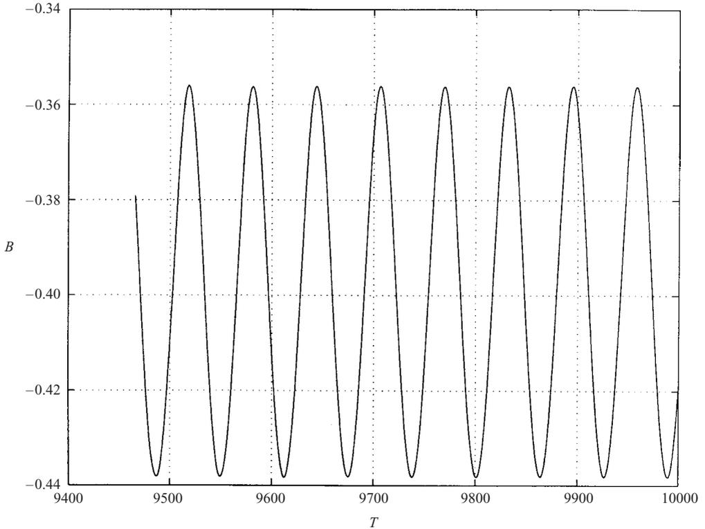
FIGURE 4. The finite-amplitude periodic solution for  $G = 1$ ,  $H = 0.1$ ,  $\omega = 0.1$ ,  $\mu = 0.01$ . The solution is shown for the last 600 time units of a run of length  $T = 10000$ . The solution has settled into a limit cycle with a period equal to the period of the oscillating shear.
