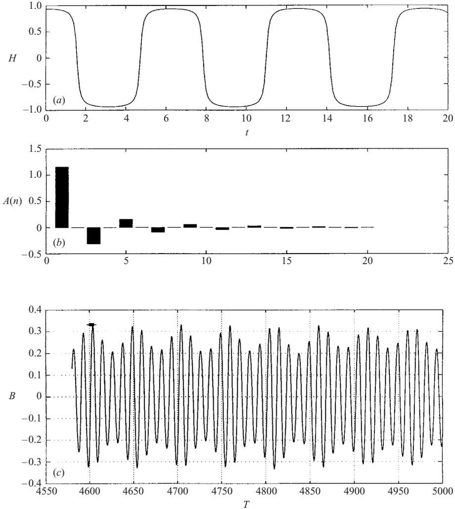
FIGURE 14. An example of the response for  $G < 0$ ,  $H < 1$  of parametric instability for a periodic  $H(t)$  which is not harmonic. (a) The function  $H(t)$  is periodic and nearly a series of step functions. (b) The amplitude  $A(n)$  of the cosine series representing  $H(t)$ . (c) The response of the perturbation amplitude as a function of time. The response is qualitatively similar to the response of figure 11 but the added harmonic content of  $H(t)$  has rendered the solution aperiodic.
