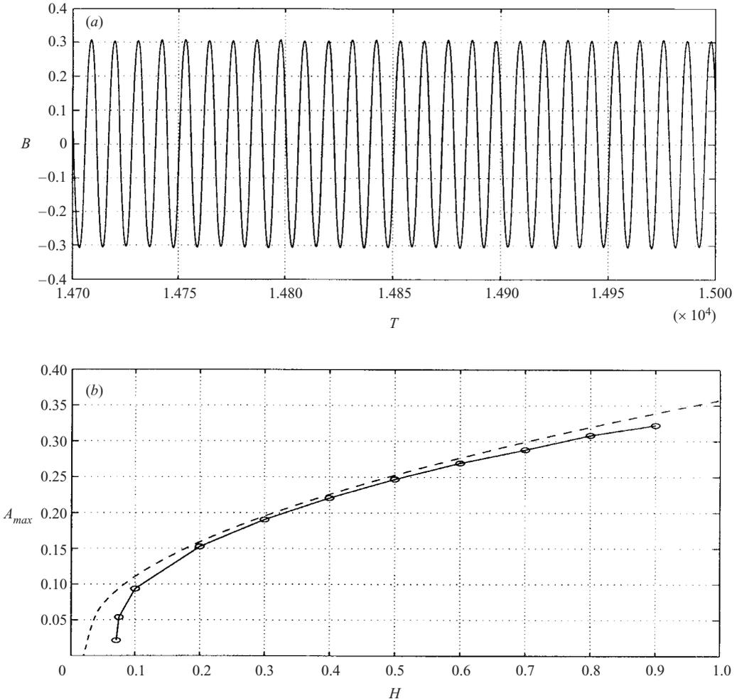
FIGURE 11. For the subcritical parametric instability at  $\omega = 1.1303$ ,  $\mu = 0.01$ ,  $G = -1$ . (a) The periodic solution for  $H = 0.8$ . (b) A comparison of the analytical prediction given by (6.11a) (dashed curve) and the direct integration of (3.13a, b), indicated by the circles and joined by the solid line.
