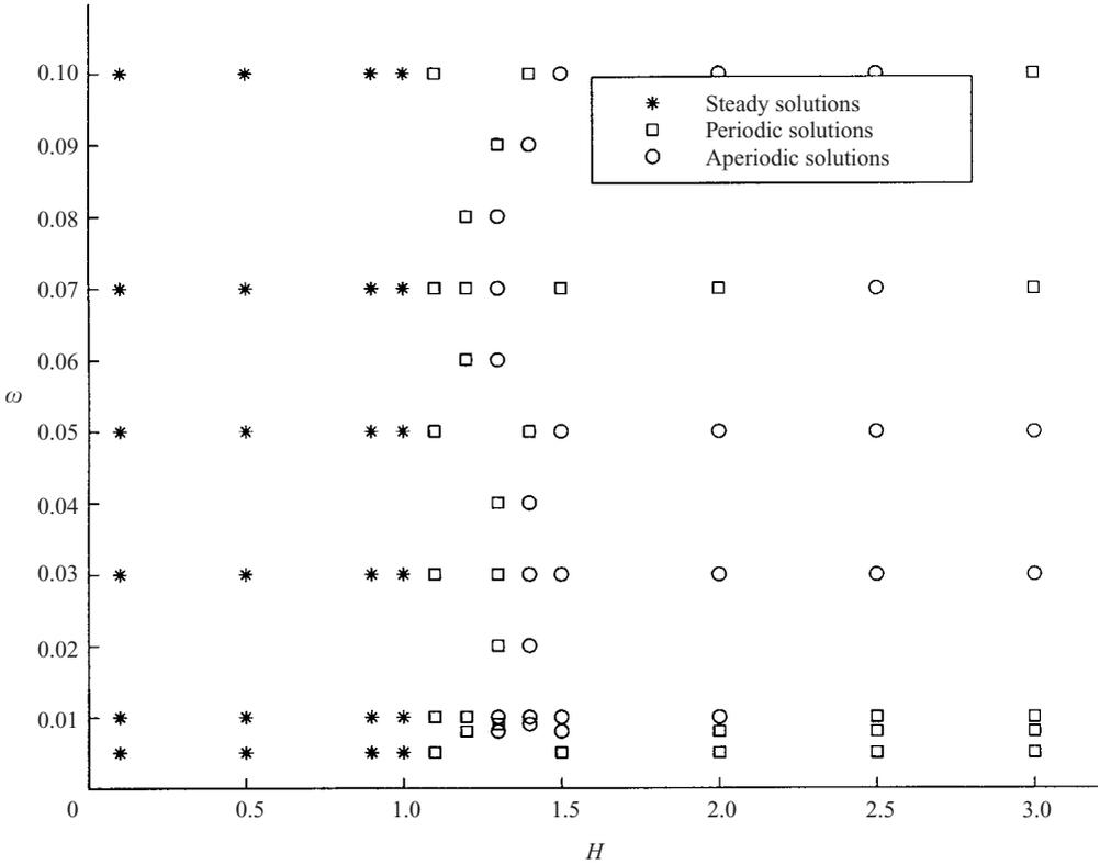
FIGURE 8. A regime diagram for  $G = -1$  in the  $(H, \omega)$ -plane. Values of  $\omega$  are restricted to values  $< 0.1$ . Larger  $\omega$  are discussed in § 5. Squares denote periodic solutions while open circles denote aperiodic solutions. Asterisks denote solutions that tend to zero for large time.
