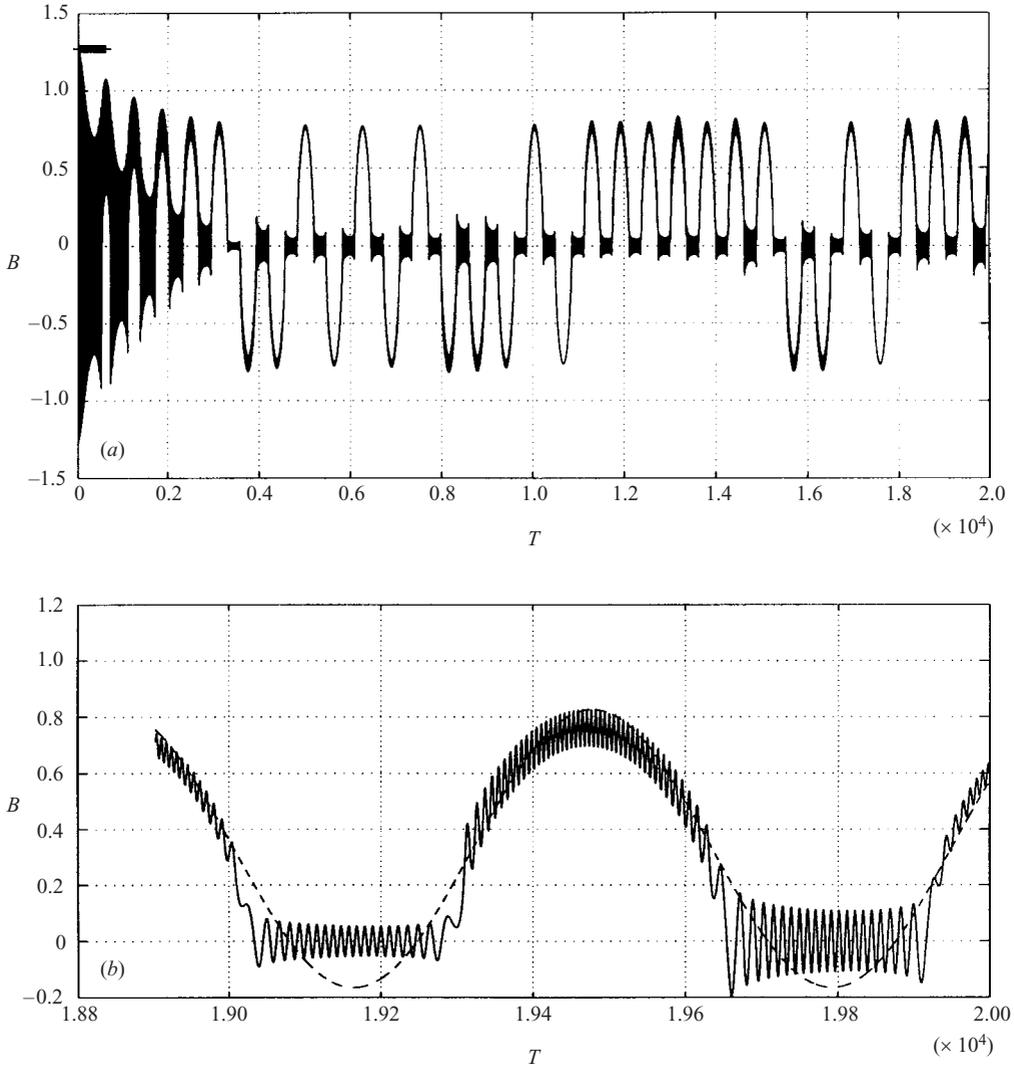
FIGURE 7. The aperiodic solution for  $G = 1$ ,  $H = 1.5$ ,  $\mu = 0.001$ ,  $\omega = 0.01$ . (a) The complete time history. (b) A detail of the last 5% of the calculation. The dashed curve indicates the overall value of the supercriticality. For small  $\omega$  the solution grows during periods of positive  $\delta$ .
