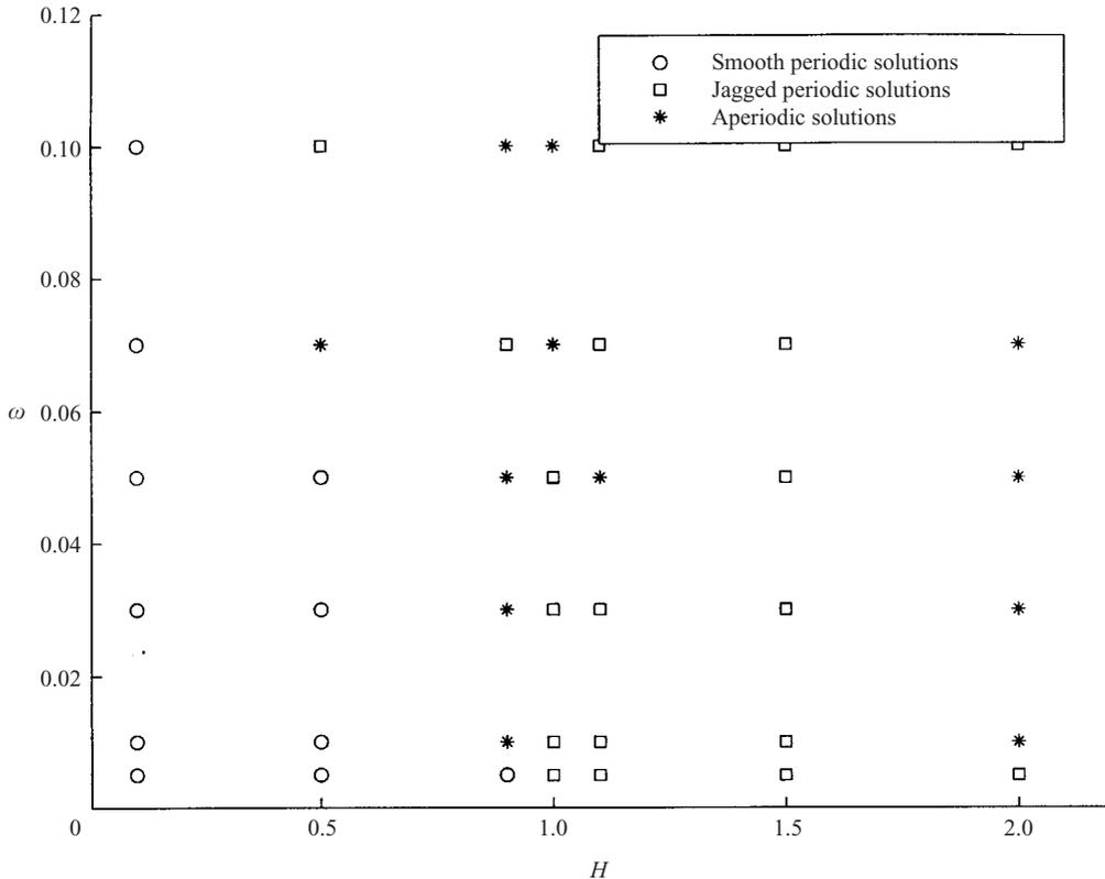
FIGURE 3. The regime diagram in the  $(H, \omega)$ -plane constructed for the case  $\mu = 0.01$  and  $G = 1$ . Three qualitatively different behaviours are noted in the figure. Smooth periodic solutions with the period of the shear's oscillation are denoted with circles, essentially periodic but ragged oscillations are denoted by squares, and aperiodic solutions with broad spectra with no sharp peaks are denoted by asterisks.
