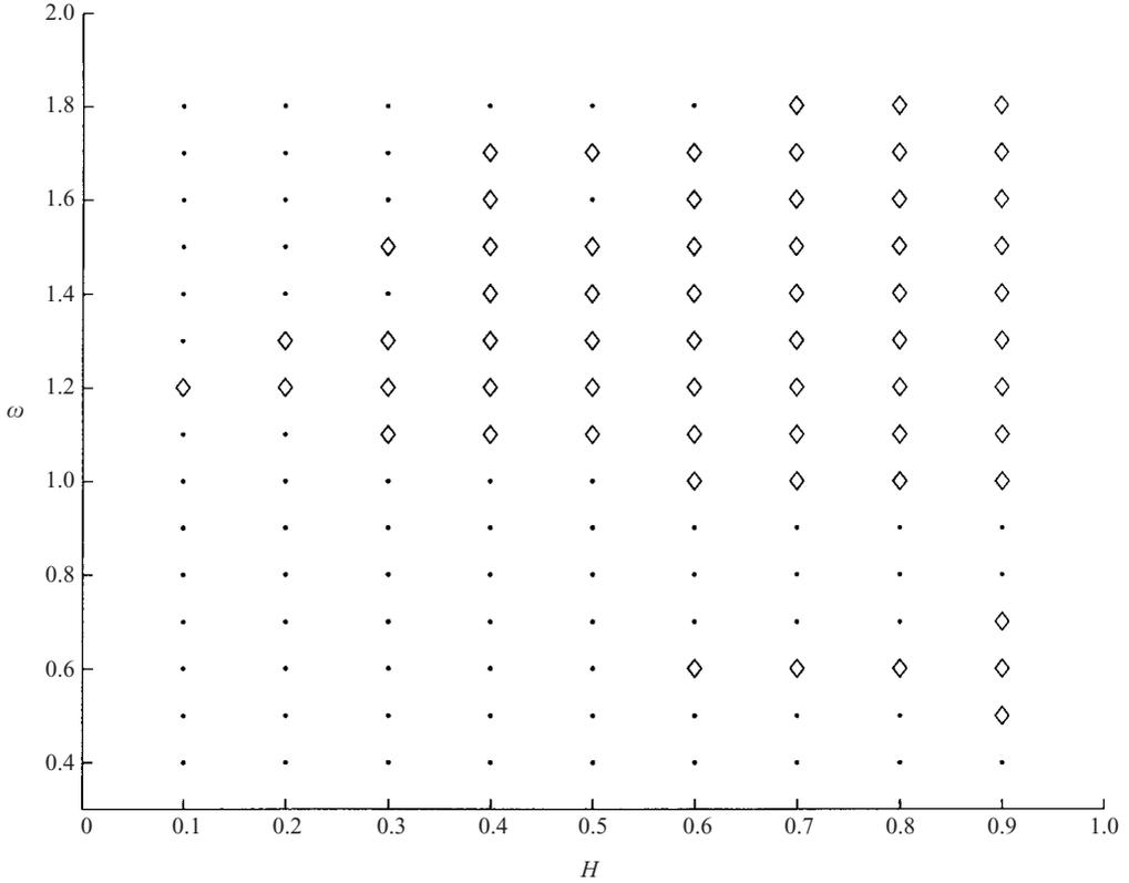
FIGURE 12. The regime diagram for  $G = -1$ ,  $H < 1$  for  $\omega$  in the range of the frequencies subject to parametric instability. The diamonds denote periodic solutions and the small dots solutions with zero amplitude.
