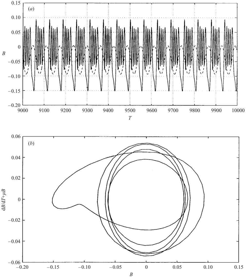
FIGURE 9. The solution for  $G = -1$ ,  $H = 1.1$ ,  $\mu = 0.01$ ,  $\omega = 0.1$ . The time-averaged shear is stable and the flow experiences brief periods of supercriticality. (a) Time history of the solution. Note the dashed curve, indicating that  $\delta$  is greater than zero only for small intervals of time. (b) Phase plane indicating the periodicity of the solution.
