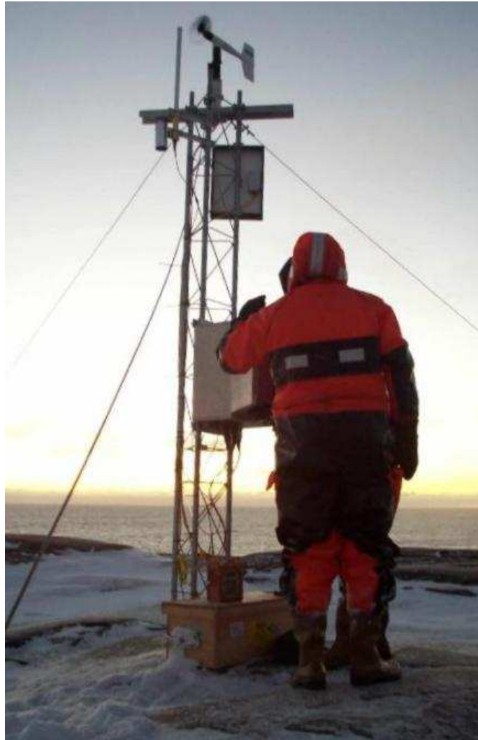
Figure 22: The photo shows the AWS station used at Kirkwood Island, equipped with an R. M. Young wind monitor, air temperature, relative humidity, and barometric pressure sensors, an electronics controller, and ARGOS telemetry link to AWSP mounted on an 8-ft tower.
