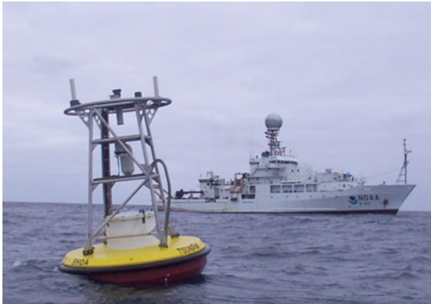
Figure 42: The surface buoy portion of the DART mooring
