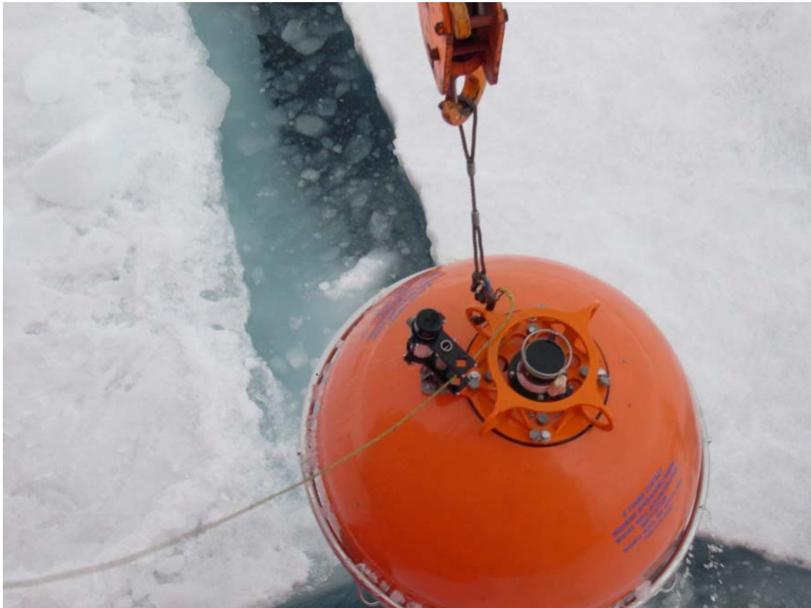
Figure 5. Top flotation sphere being recovered using the ship's crane.
