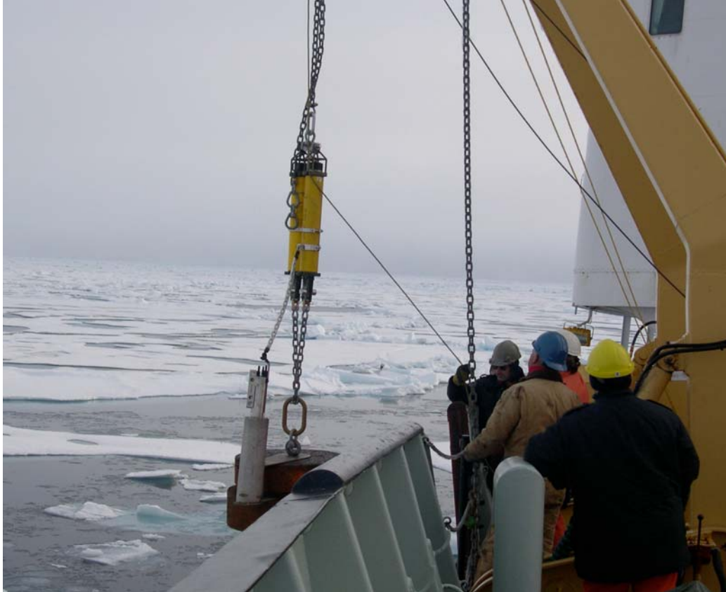
Figure 9. Lowering the anchor, BPR, and releases during anchor first mooring redeployment.
