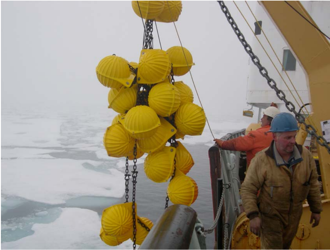
Figure 8. Cluster of glass floats comprising the backup buoyancy being recovered.
