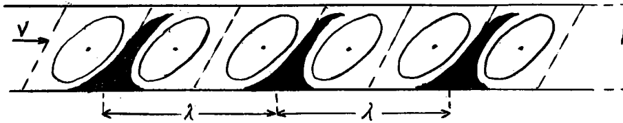
Fig. 49 Schema of cellular eddies in very slow movement of translation; the crests of smoke slope forward under action of the general current.
