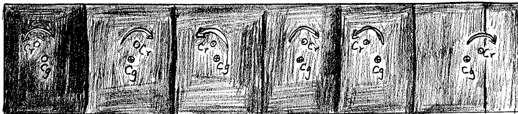
Fig. 99 Experimental eddies of two dimensions in a layer of air with diffused tobacco smoke. The geometric centers C_g of the cellules do not coincide with the centers of rotation C_r . h = 65 mm.
