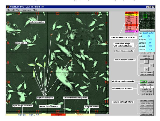
The DIGITIZER Main Window shown here contains a portion of a typical scanned image and several digitized samples, along with various control buttons, information boxes and edit boxes. Detailed descriptions of these elements are presented in subsequent sections of this document.
