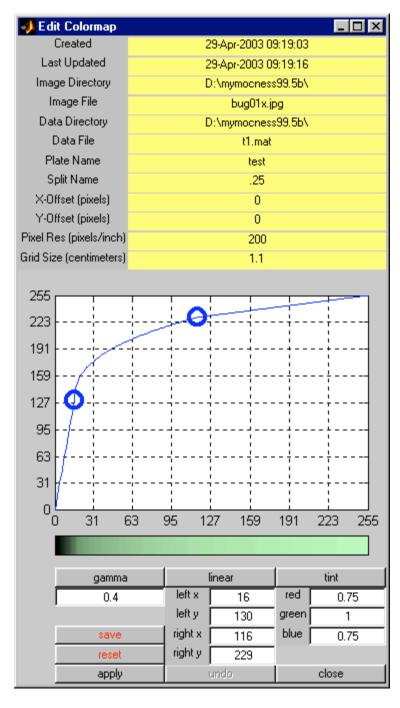
The image "exposure curve", which is the relationship between the byte value of a particular pixel appearing in the image file and the screen color used to display that pixel,
