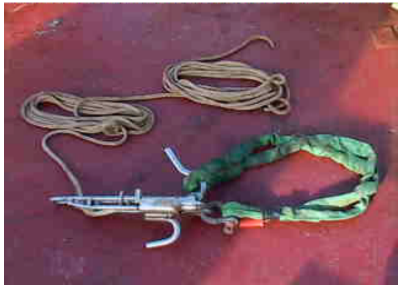
Figure 13. Brailer release hook and Lift All sling
