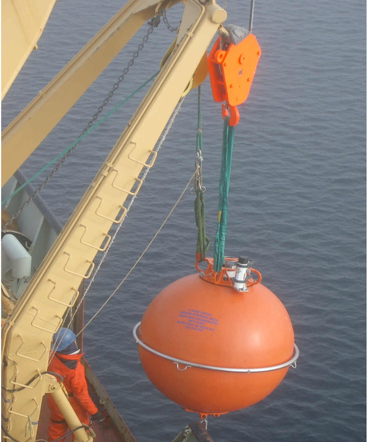
Figure 14. Sling detail: sphere deployment
