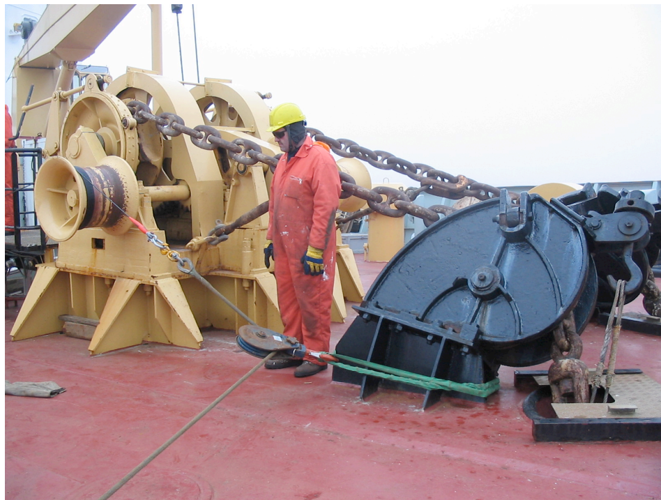
Figure 9. Fair lead block and stopper line
