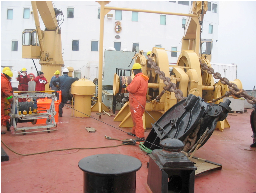
Figure 11. Wire fairlead windlass capstan to tension cart
