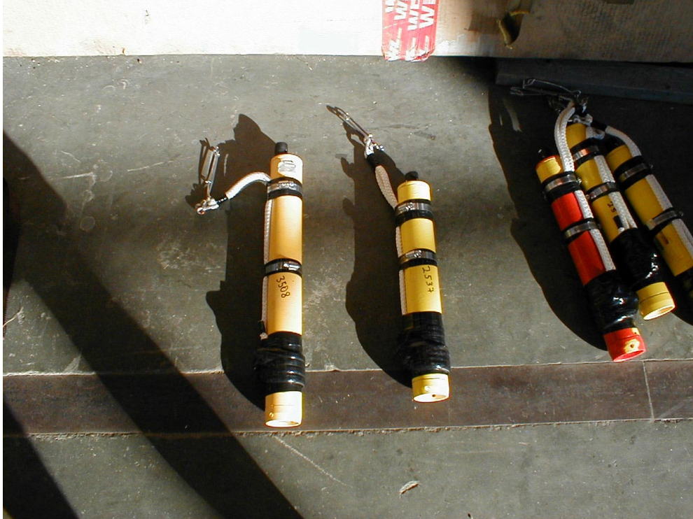
Figure 8: Photograph of the rigging method for Brancker temperature loggers used on the three-dimensional array.
