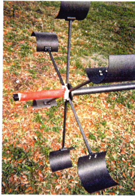
Figure 2-2. Detail of prototype vanes. The axial tube contains the drop weight.
