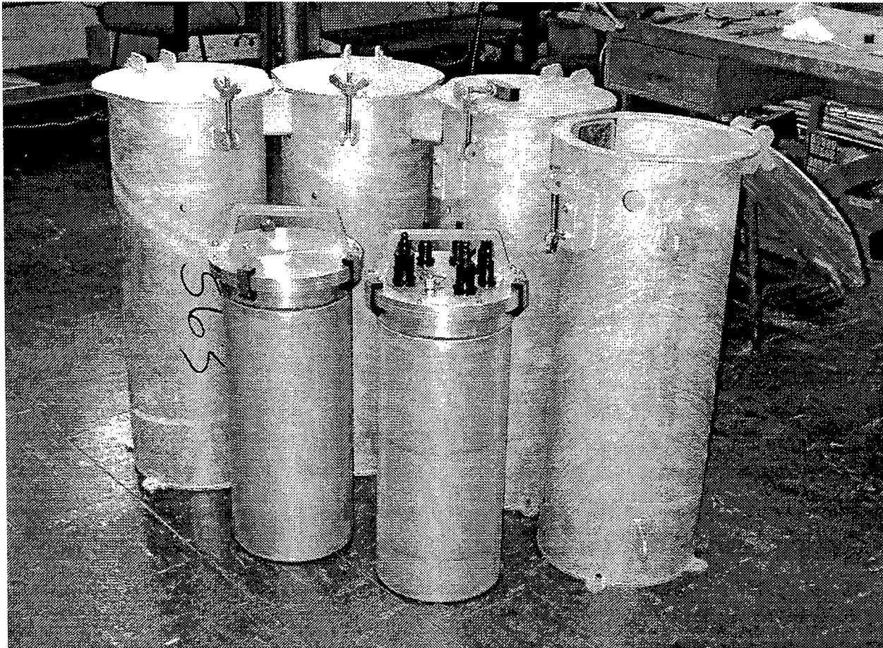
Figure 6.5. The battery pressure case (front left), the electronics pressure case (front right) and the mounting silos (rear) for the motion package on the top of the fish cage central spar.
