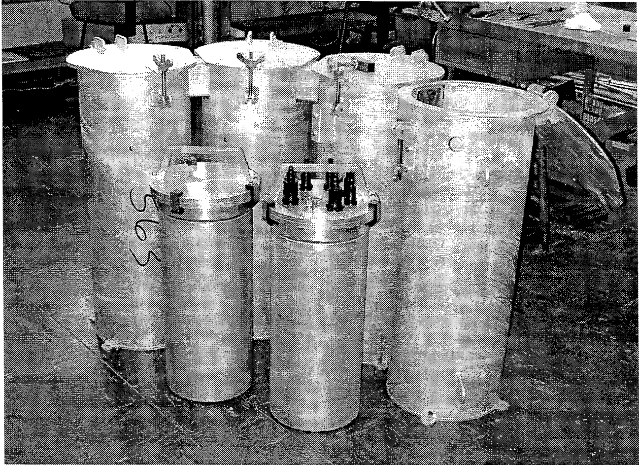
Figure 4.28. Four silos built for the top of the fish cage to hold two battery pressure cases (one shown front left) and motion package electronics pressure case (front right). The silos were to be bolted to the top of the UNH-OOA fish cage in holes drilled during servicing in summer 2000. They are connected at the top with square metal tubes to allow cables to be run freely between the electronics and antennas, and down to sensors mounted on the fish cage. The second silo from the left contains the mounting hardware for the telemetry module (Figure 4.27) and the cables from the fish cage to the motion package. The antenna bolts to the two tabs on the silo on the right, and a solar panel mounts on standoffs seen on the top of the right two silos. The solar panel provides power to the battery used by the load cell telemetry package to relay data from the four load cell recorder on the Northeast mooring leg to shore [see Appendices 9.2.4, 9.5.1, 9.5.2 and 9.5.3].
