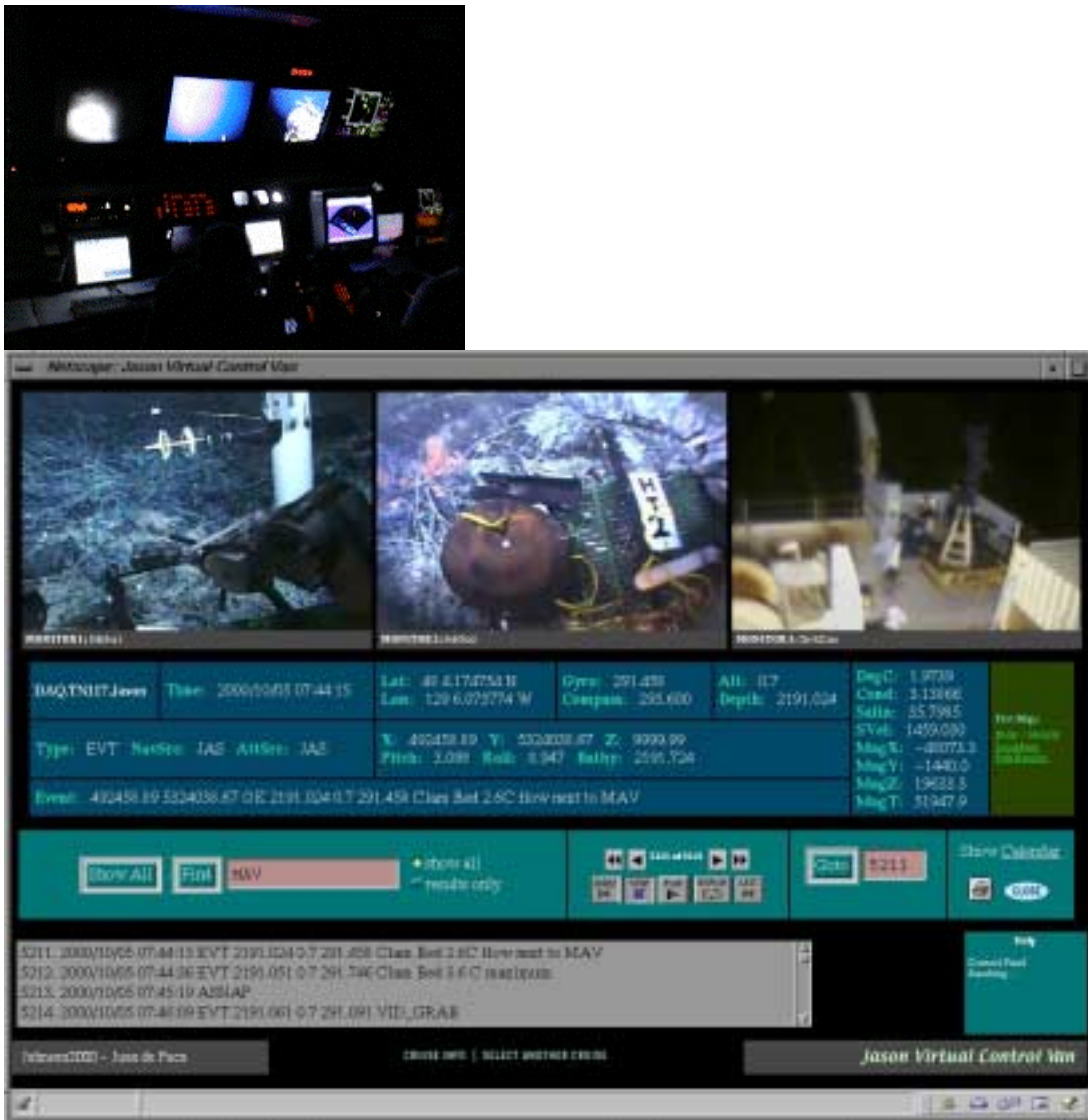
Figure 2-4: Photograph of inside the Jason Control Van (upper image), The Jason Virtual Control Van (lower image). The Virtual Control Van enables users to play the data back and forth in time and search for items by keywords, dates/times, and events.
