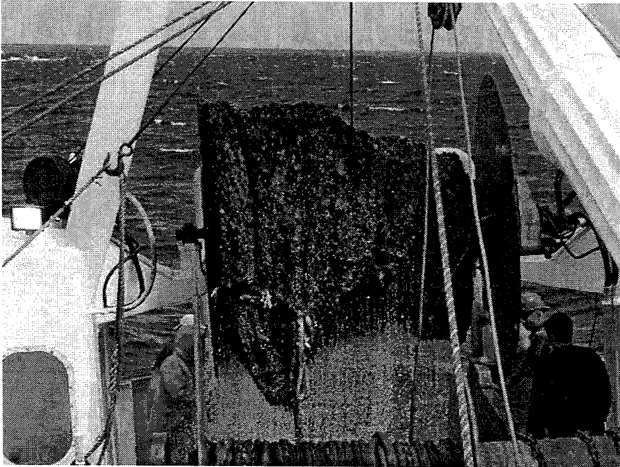
Photo P001240 - winding the northern fish cage net onto the Nobska aft net reel. The whole operation from pickup of the buoy to net wound upon the net reel took about two minutes.
