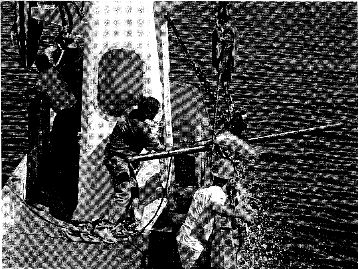
Photo P001189 - Mat Stommel (left) cutting chain wrapped around anchor while Will Ostrom (right) keeps water on line so that sparks from the cutting torch will not burn line holding the anchor chain for recovery on the aft fish reel.
