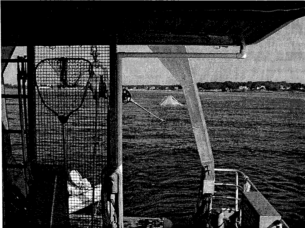
Picture 33. The fish cage can be seen being towed behind the Gulf Challenger in the Piscataqua River. The towing cable seen was attached to the bridle lines on the fish cage on one end and a load cell on the other. The load cell is in the dark open frame seen at the left end of the tow rope above the deck. The other end of the load cell was restrained by a line running over a block in the A-frame and down to the winch and cleat on deck.
