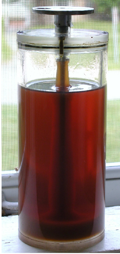
Figure 12: A photograph of the rod climbing effect. The device consisted of a rod immersed in the lower, darker fluid. As the rod is rotated, normal stresses cause a fluid column to rise near the rod.
