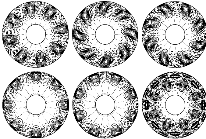
Figure 3: The streamfunctions r \sin \theta \partial_\phi v in the equatorial plane illustrating the sequence of transitions for the same parameters as Fig. 2 and values of \tau = 5, 950, 1500, 6 \cdot 10^5, 8 \cdot 10^5, 3.5 \cdot 10^7 .
