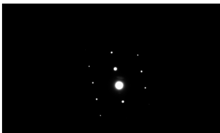
DEP Electron diffraction Showing crystalline structure
