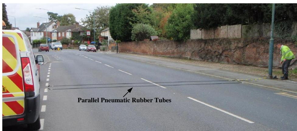
Figure 7.2 parallel pneumatic rubber tubes for automatic traffic volume surveys
