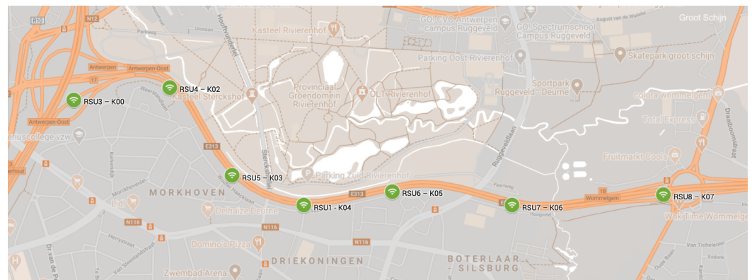
Figure 5. The positions of the Road-Side Units (RSUs) deployed along the E313 highway.
