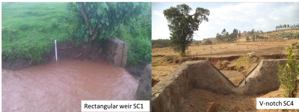
Fig. 3. Setup of weirs and diver/staff gauge at the outlet of the sub-catchments.
