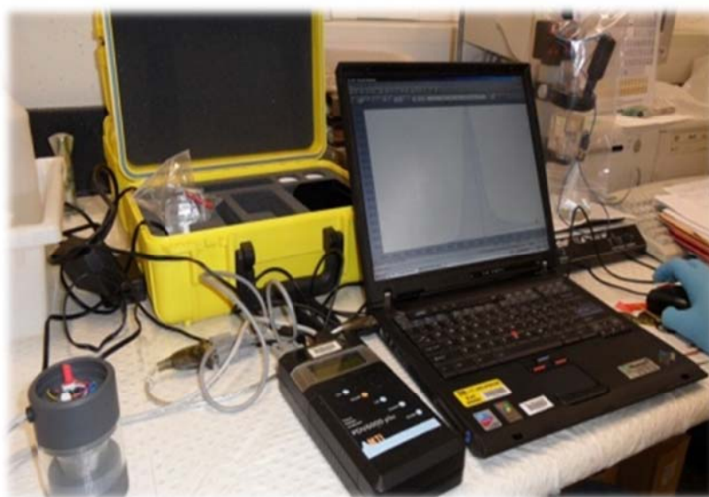
Figure 6. PDV6000plus portable voltammetric analysis instrument set up in conjunction with a laptop computer. An electrochemical cell is shown at bottom left corner.
