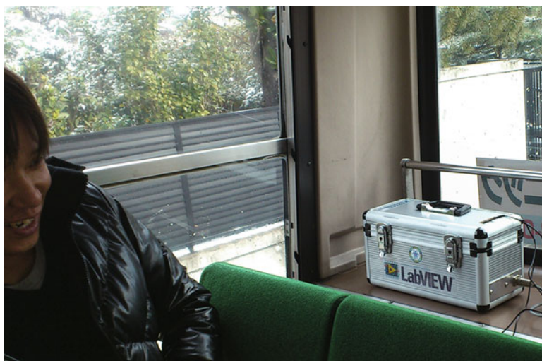
Fig. 10.7 KURAMA-II under the field test on a local bus
