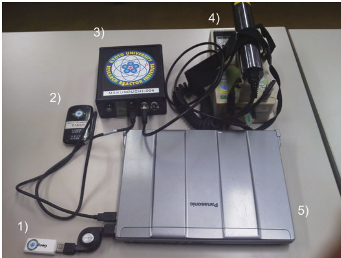
Fig. 10.2 The in-vehicle part is compactly composed of mostly commercial components. (1) GPS unit, (2) 3G mobile Wi-Fi router, (3) MAKUNOUCHI, (4) NaI survey meter, and (5) PC
