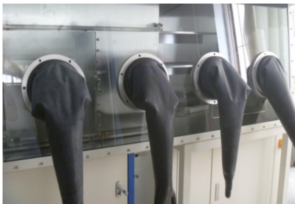
Figure 13: Picture of the Glove box of the Organic thermal evaporator housed in ESRI's cleanroom.
