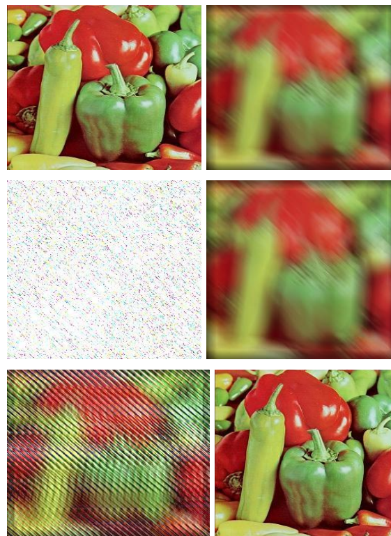
Fig. 2. Application on Pepper (jpg. format) RGB image with degree of blur 27*27. Top Left: Original. Top Right: Blur image PSNR=17.02, RMSE=35.95. Middle Left: A.F, PSNR=7.03, RMSE=113.45. Middle Right: G.F, PSNR=17.02, RMSE =35.94> Bottom Left: M.F, PSNR=11.79, RMSE =65.65. Bottom Right: Proposed, PSNR=46.23, RMSE=1.24
