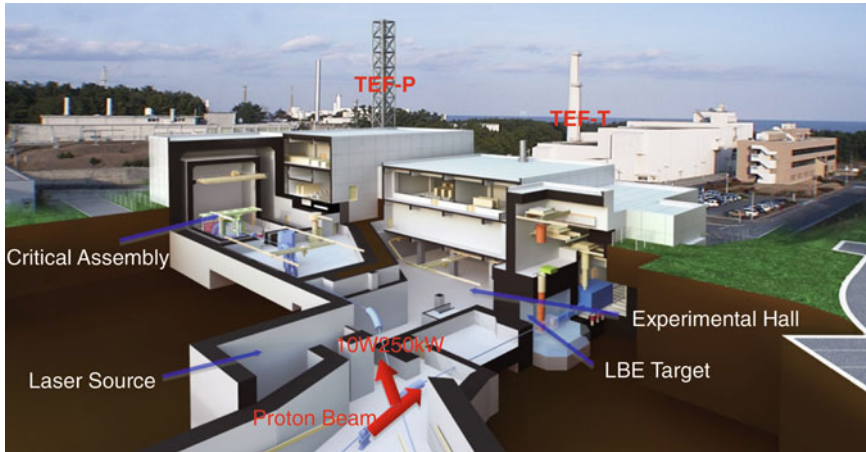
Fig. 8.1 Transmutation Experimental Facility
