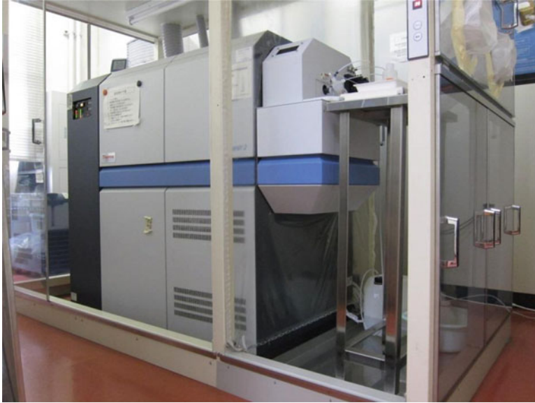
Photo 6.1 High-resolution inductively coupled plasma mass spectrometry (HR-ICP-MS) introduced in JAEA for the measurement of fission product nuclides [6]
