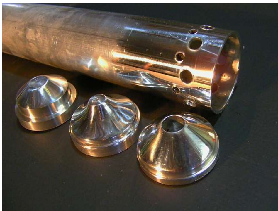
Figure 5. Manufacture of Cone-shaped Baffles.
