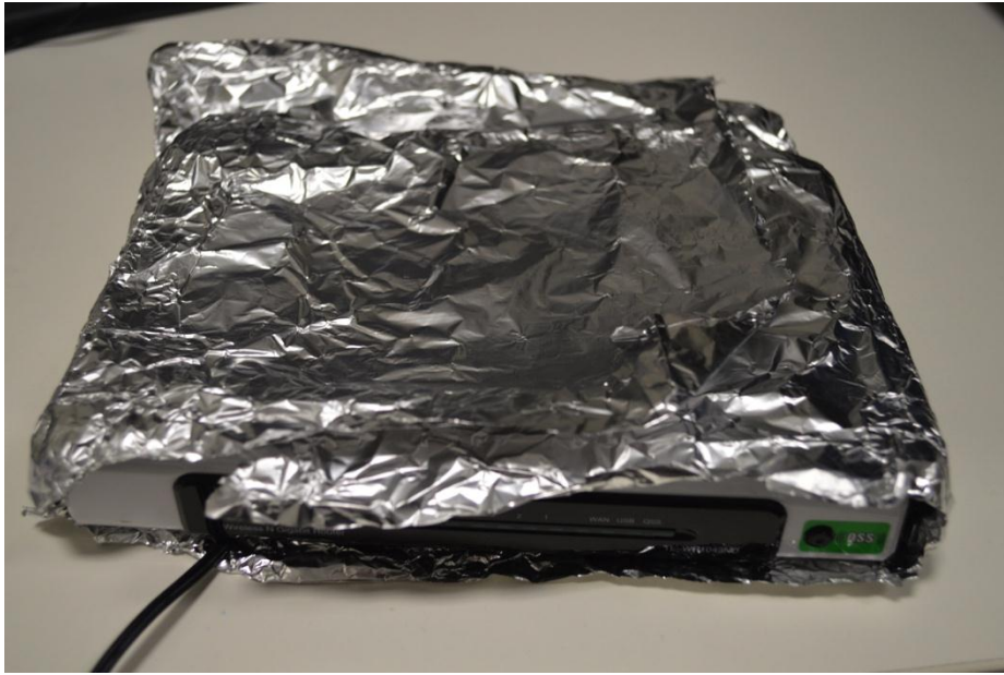
Figure 6 - TP-Link TL-WR1043ND covered in aluminium foil with large opening at the front
