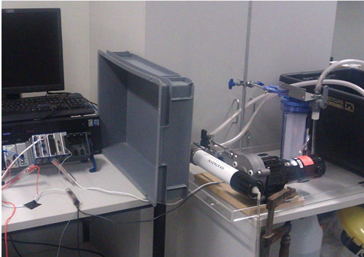
Figure 2.2 - Experimental setup with the RO unit and the data acquisition system.
