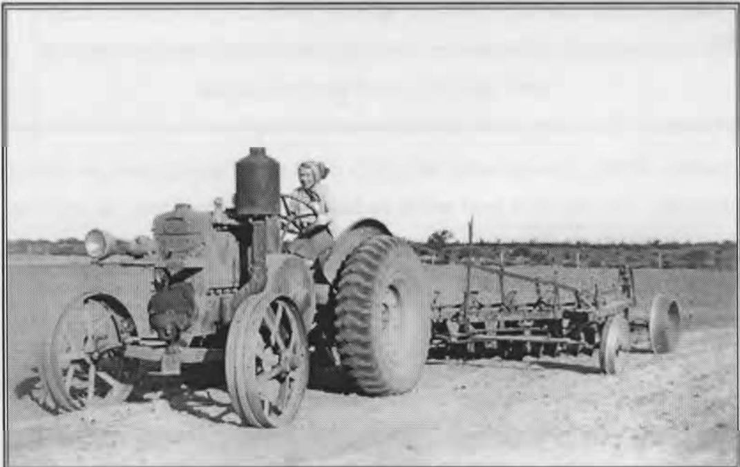
Ebba Wassard pulling a disk plough with the Lanz HR5 Bulldog , which had a top speed of 3.5 mph (5.6 kph, less than 100 metres a minute). May 1946.
