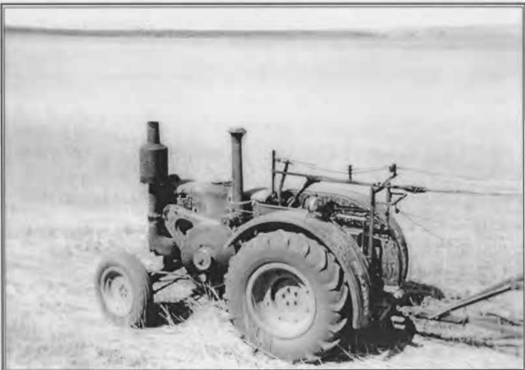
The KL Bulldog rigged up with remote controls (steering, clutch and brakes) to the harvester. December 1955.
