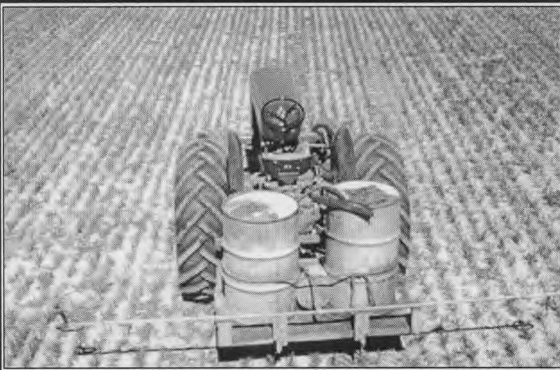
Two 44-gallon drums fed the spray arms on the back of the Massey Ferguson MF65 in August 1961.
