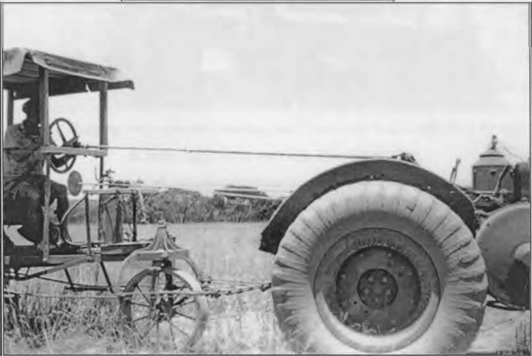
Lanz HR5 tractor with remote steering, clutch and brake, controlled with rods and universal joints from the Sunshine AL harvester. December 1947.
