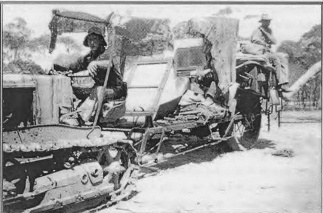
The operator of the WA Sunshine harvester, under the hessian shade, controls the comb height and choke cutter. At his feet are sacks ready for bagging. The wheel under the box is the drive wheel. Summer 1930.
