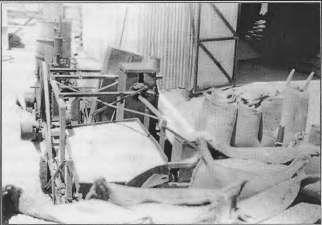
Wheat from the tray of the old Chevrolet truck is poured into the hopper of the Hannafords grader, pickled, graded, bagged, sewn up and stored in the new shearing shed at right. 12th December 1948.
