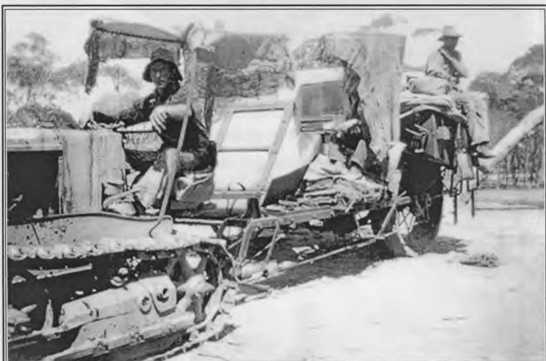
Hector Rhind driving the Holt 2-ton, with hands resting on the steering horns. The two passengers operate the Mackay Sunshine WA harvester. Harvesting at Kulja, 13th November 1930.
