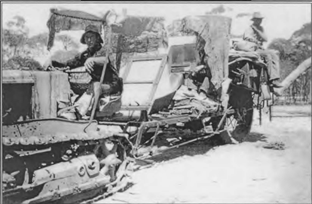
Hec pulling a Mackay Sunshine WA harvester with a Holt 2-ton crawler. The two men on the harvester control the comb height and bag the wheat. Nov. 1930.
