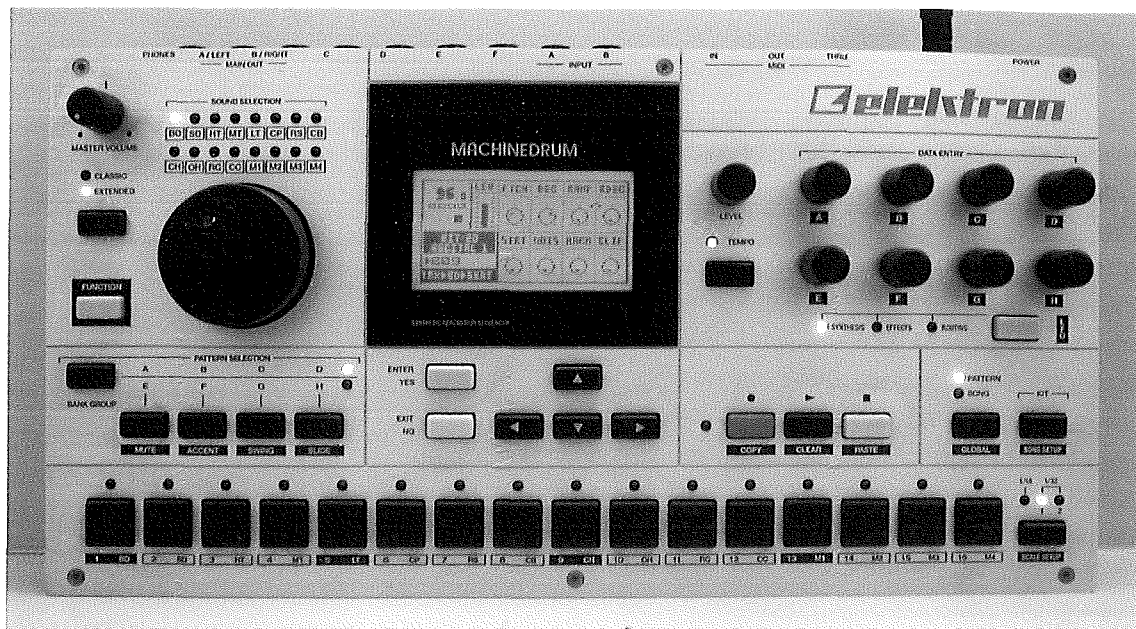
Figure 4. The Elektron Machinedrum SPS-1. The row of sixteen buttons along the bottom is used for entering pattern data, while the other knobs and buttons control various functions and sound parameters.
