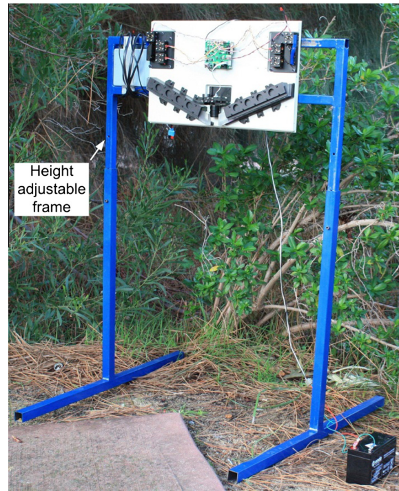
Fig. 12. Illustration of the static experimental setup used for plant spectral reflectance measurements.
