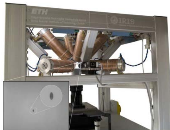
Fig. 2.11. The Octomag system contains eight soft-magnetic-core electromagnets and in the central space of eight electromagnets is the untethered microrobot [11].
