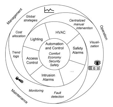
Figure 1: Integrated Building Automation System, adapted from Kastner (2005)
